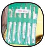
Don Sobel: special tool for screws on plates. And a set of broaches for oil sinks. He suggested cutting them in half and using halves in a pin vice.
